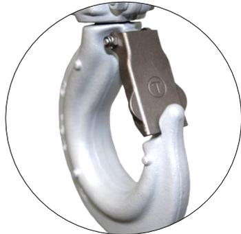
The entire hook fitting has been protected using corrosion protected or stainless steel fixtures and fittings. Our latest latches incorporate a new wing design making them easier to operate in the operation area (e.g. wet gloved hands for offshore or subsea use).
