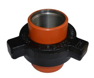
Recommended for air, water, oil, gas or mud service to 6,000 PSI NSCWP. This union has a replaceable lip-type seal ring of Buna-N specifically designed to minimize fluid flow turbulence. Lip-type ring provides a pressure seal and protection for metal-tometal seating surfaces. Smaller and lighter than Fig. 600 unions and are recommended for manifold and truck mounting where size and weight are critical.
