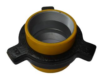
Recommended for air, water, oil, or gas service to 1,000 PSI NSCWP. Standard subs are threaded for API line pipe and are Weco interchangeable. Also available with butt weld ends.
