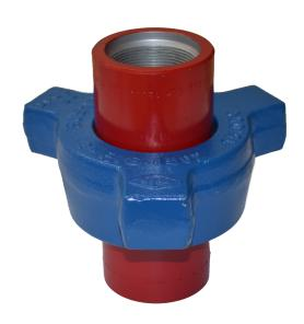
Recommended for air, water, oil, gas and mud service to 15,000 PSI NSCWP. This union has a replaceable lip-type seal ring of Buna-N specifically designed to minimize fluid flow turbulence. The lip-type ring also provides a pressure seal and protection for metal to metal seating surface and are recommended for manifold and truck mounting or other installations where high pressure is encountered.
