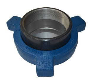
Recommended for air, water, oil or gas service to 2,000 PSI NSCWP. A Buna-N 'O' ring is mounted on the plain sub to provide an additional seal. Subs and nuts of the Fig. 206 union are interchangeable with the Fig. 200 union. Standard subs are threaded for API line pipe. Sizes of 2" and above also available with butt weld ends. connections.
