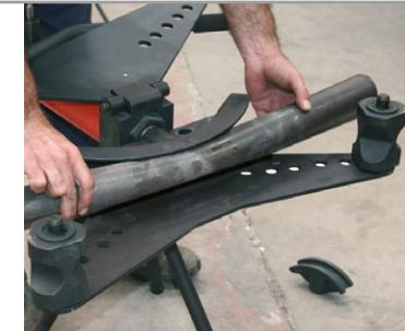
2. The double plate provides optimum consistency and safety during its operation.
